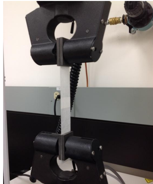
Fig. 4: LJSS sample in the tensile tester
