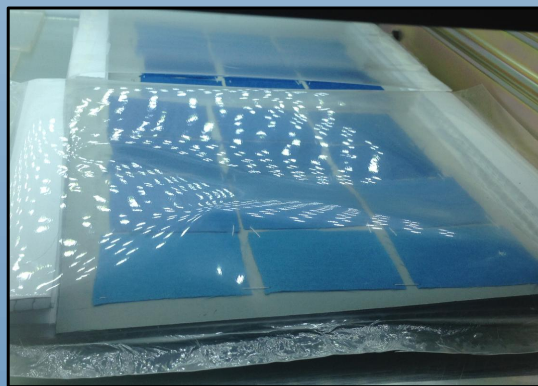
Fig. 3. Ambient and anoxic sample sets fading in the LED light chamber.
