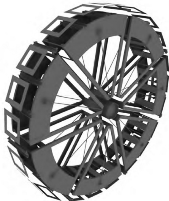
Fig. 3. Scheme of the main steel elements of the wheel. Courtesy of Volker Möllenhoff.
