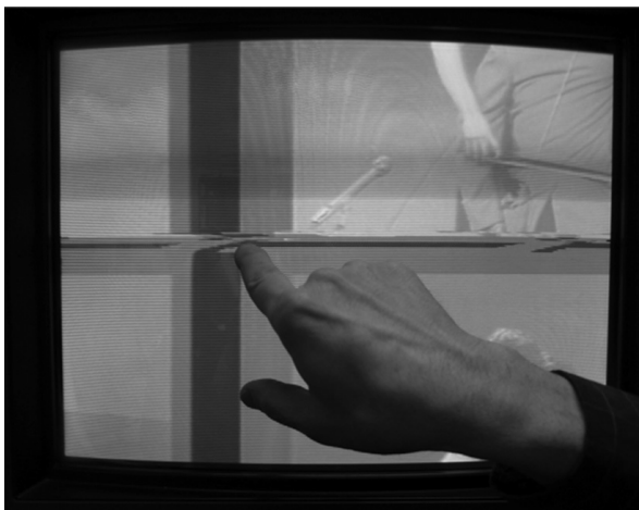
Fig. 4. Illustration of head-switching point in pulse-cross display during examination and evaluation at DuArt Film & Video, New York, April 2010. Courtesy of Christine Frohnert.
