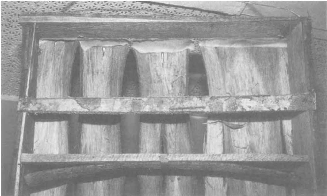
Figure 6. The rack showing tinted paper adhered to Ethafoam blocks with Rhoplex N580.
