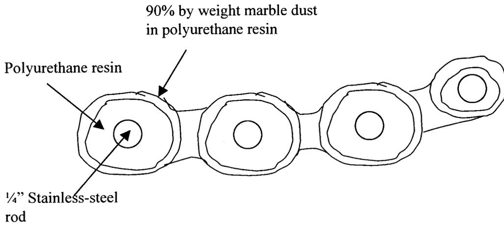
Figure 6. Cross-section of fingers of cast replacement hand.
