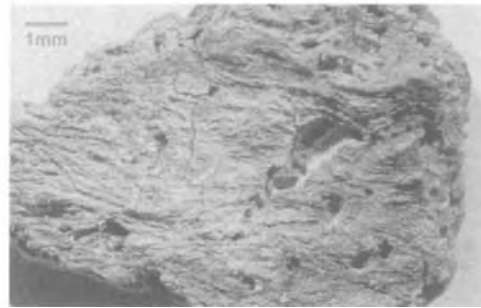
Figure 12. Concave interior surface with striations, possibly impressions of a wooden mold [AG 22A].
