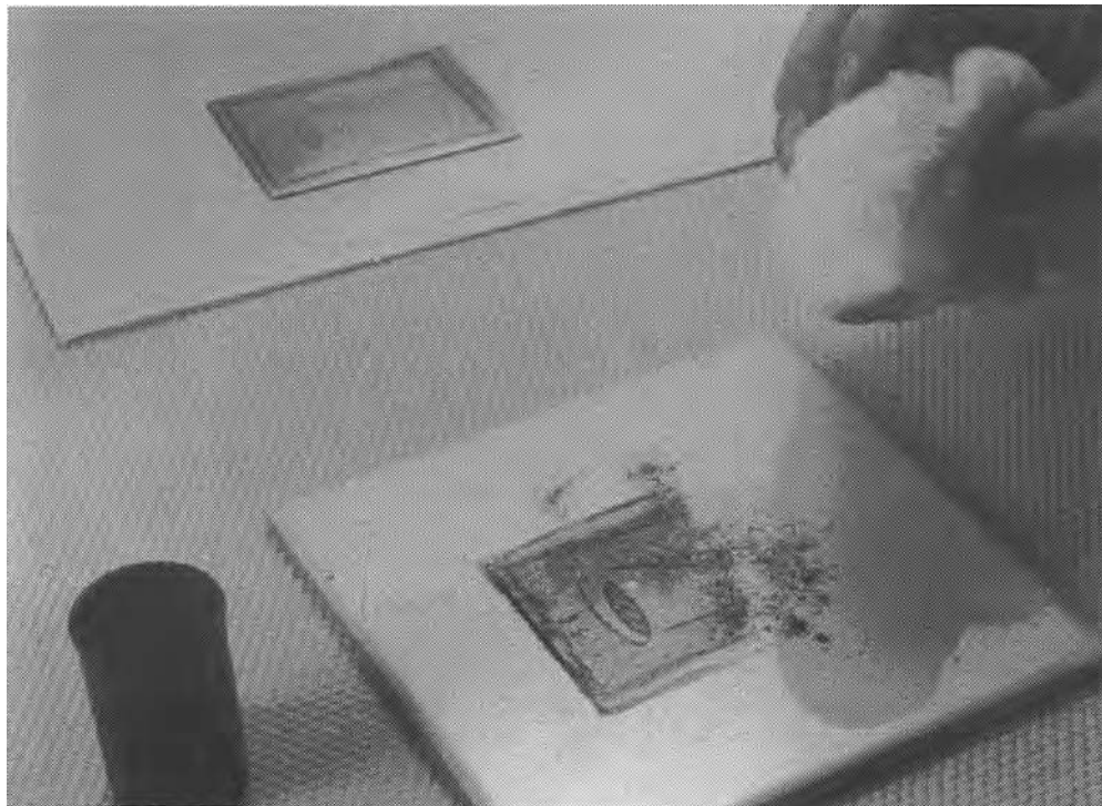
Figure 10. Dusting the oil image with ceramic pigment (from Scott 1994).
