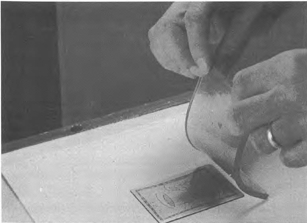
Figure 8. Application of "glue bat" to the oil laden copper plate (from Scott 1994).
