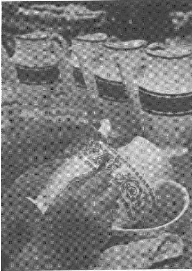
Figure 14. Application of a gum based paper design onto a pitcher (from Chandler 1968).
