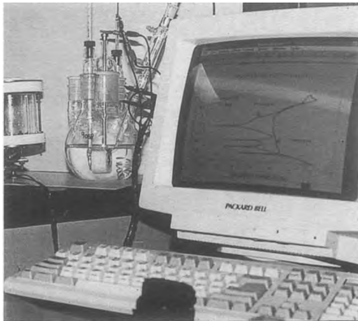
Figure 1. A typical electrochemical testing system, including a test cell containing an electrolyte, working electrode, reference electrode, and auxiliary electrode; and a computer with potentiostatic boards installed.
