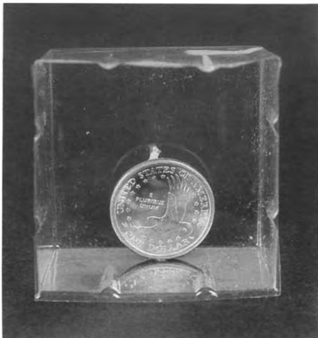
Figure 7. Coin attached with toothpick fragments before pouring of silicone rubber.
