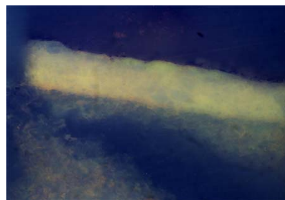
e. stained with RHOB (note positive reaction for oil as indicated by red-orange fluorescence in paint layer)
