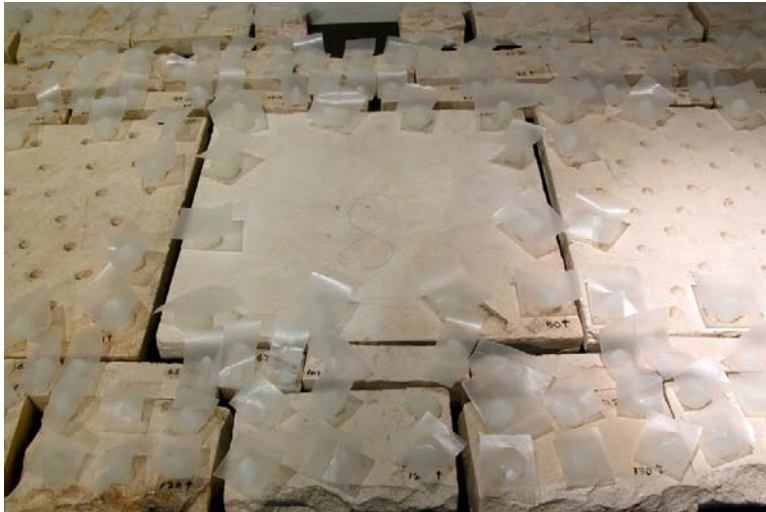
Figure 6. Wax spacers with release paper.
