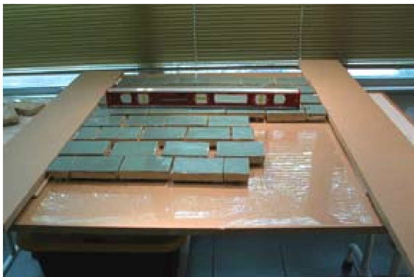
Figure 8. Leveling a row.
