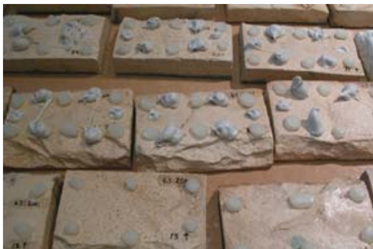
Figure 9. Epoxy piped between the wax stilts.
