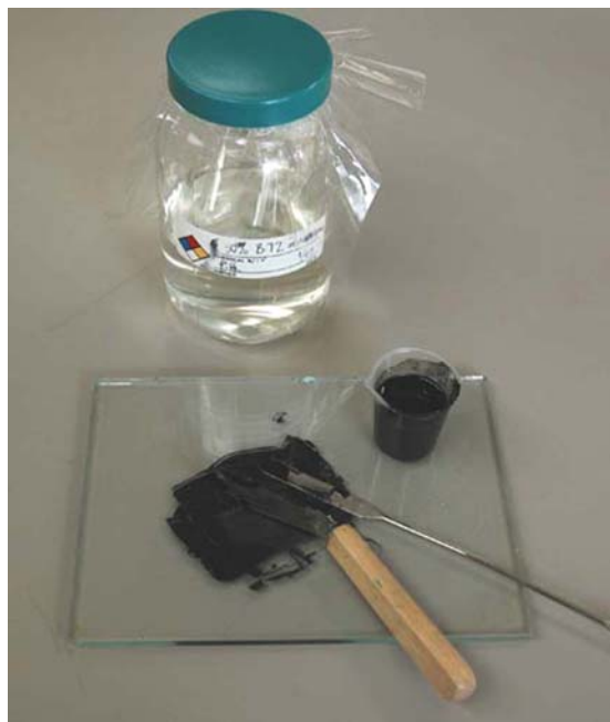
Figure 8. Dry powdered pigments are used to tone the resin to match the area of loss. The pigments should be milled before mixing to produce a homogenous film. A small amount of xylene is used to wet the dry pigments for mulling. After mulling, the pigment and xylene paste is mixed with 50% B-72 in acetone (w/v).
