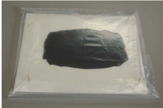
Figure 10. After casting many unsuccessful films with air bubbles, the authors consulted Stephen Koob, who recommended casting the pigmented resin on a polyethylene substrate and covering for the first 24 hours to restrict but not prevent solvent evaporation. A plastic bag works well as long as supports are used to prevent the top of the bag from touching the B-72 film. The enclosed air space creates a xylenes vapor chamber that prevents skin formation on the surface of the B-72 film during curing (Koob, 2005).
