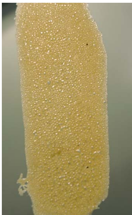
Figure 9. Unsuccessful film with air bubbles
