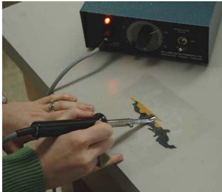
Figure 13. The cut-out sections are fused together, their surfaces smoothed, and the film thinned using a heated spatula between sheets of silicone release Mylar.
