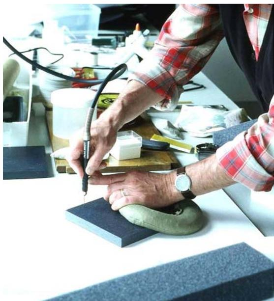
Figure 11. Packing design and travel mounts: drilling holes in foam-core for wires.
