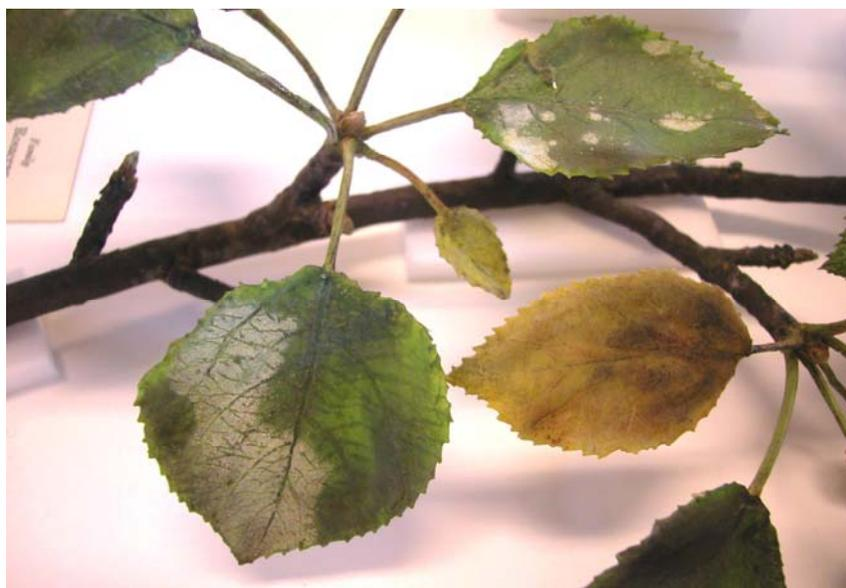
Figure 7. *Malus pumila*, Apple #609 (1933), closeup showing lead salts efflorescence.
