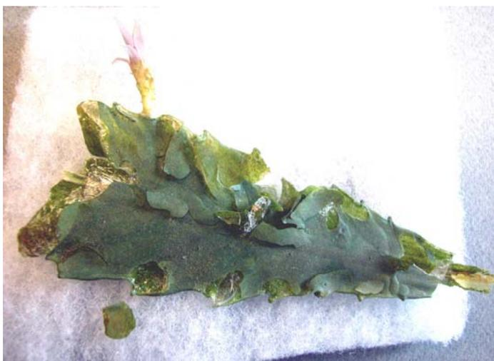
Figure 6. Cactus leaf showing surface delamination of the glass caused by shrinkage of animal glue coating.
