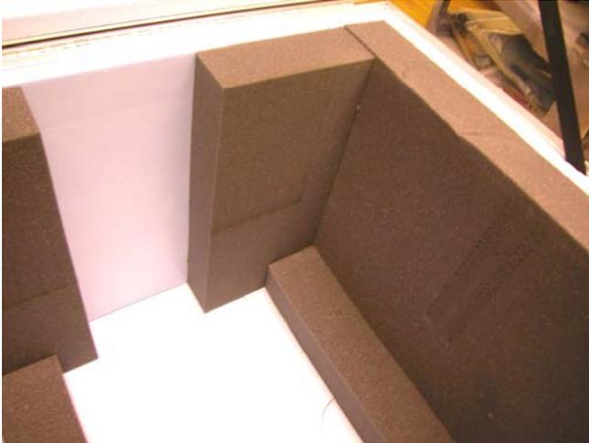
Figure 15. Outer crate showing interior foam cushioning.
