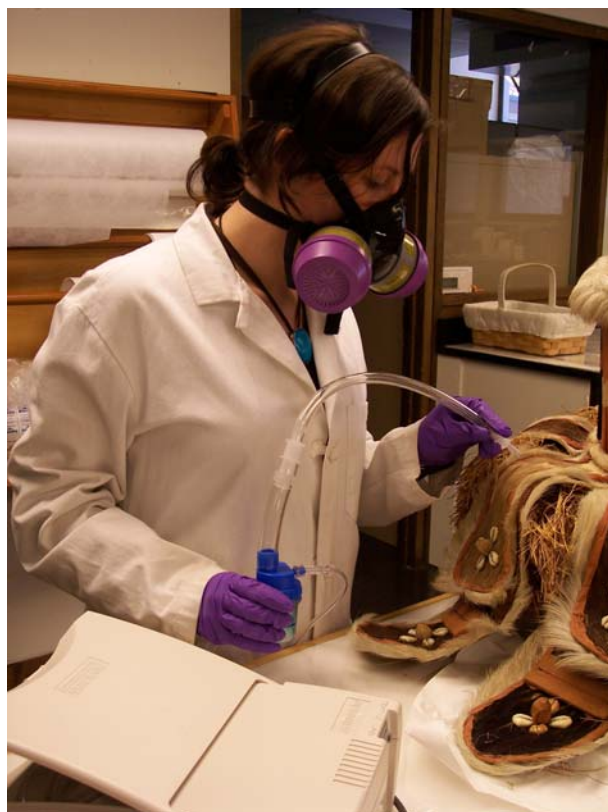
Figure 4. Mist consolidation of the hair.
