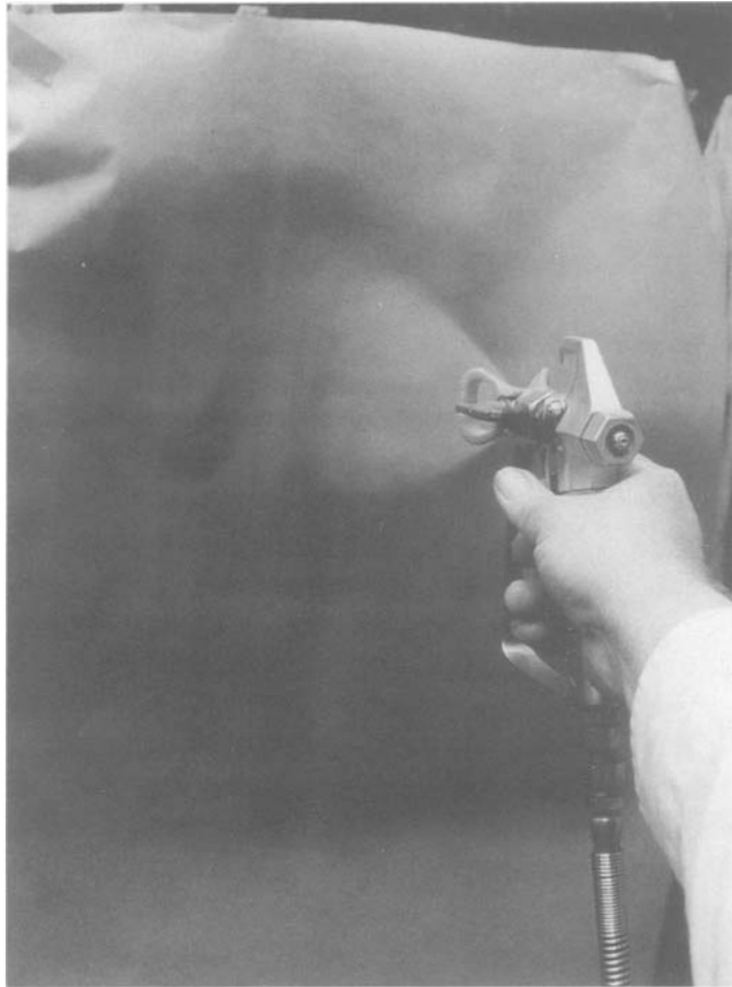
Figure 1. Test/practice application of wax using an airless sprayer. Proper material consistency, speed of application, working distance and nozzle selection allowed a smooth uniform application of wax onto a sheet a kraft paper.
