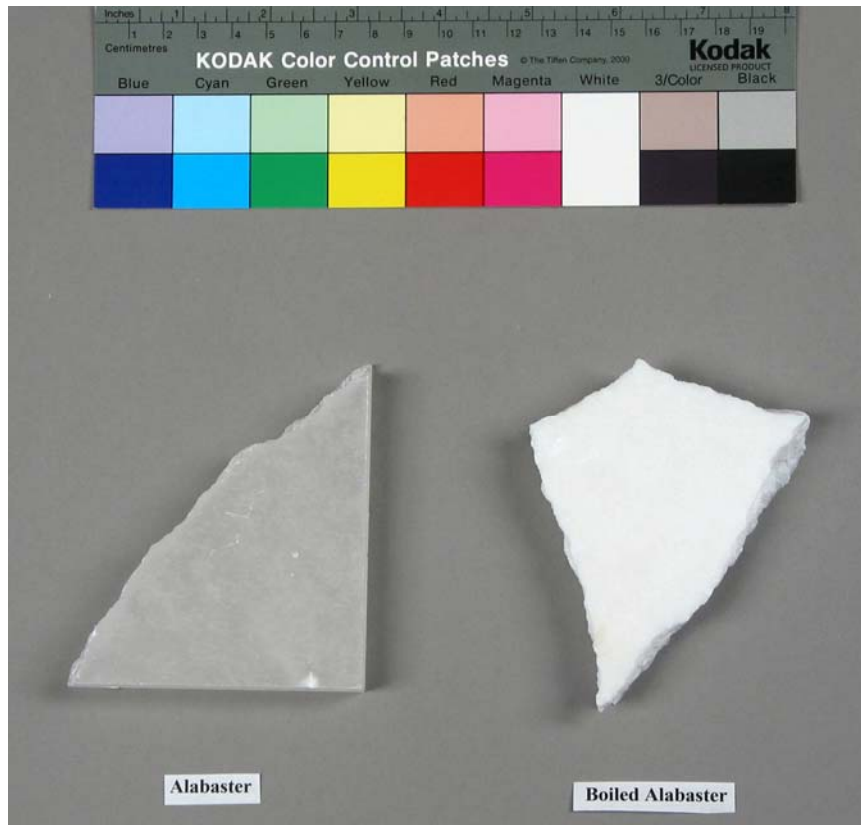
Figure 5. Test using crushed and boiled alabaster.
